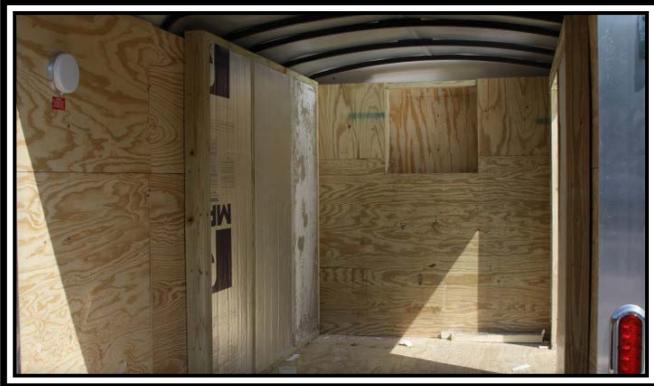
The front-end wall cutout holds the air conditioning unit.
