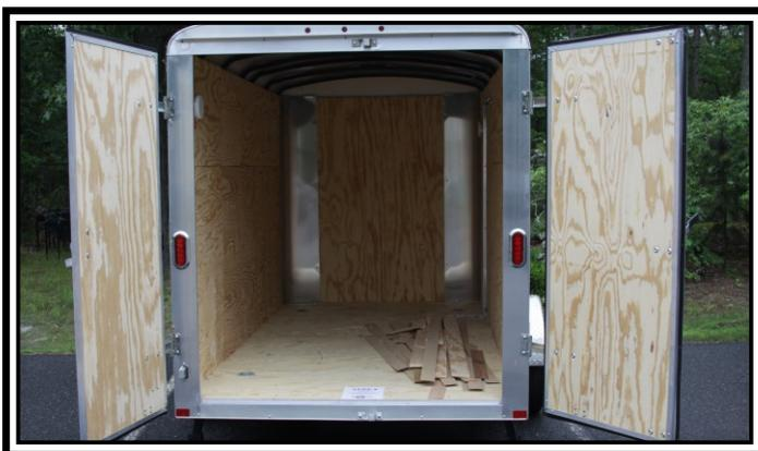
The interior plywood skin and aluminum trim pieces were removed from the front and sidewalls of the trailer.
