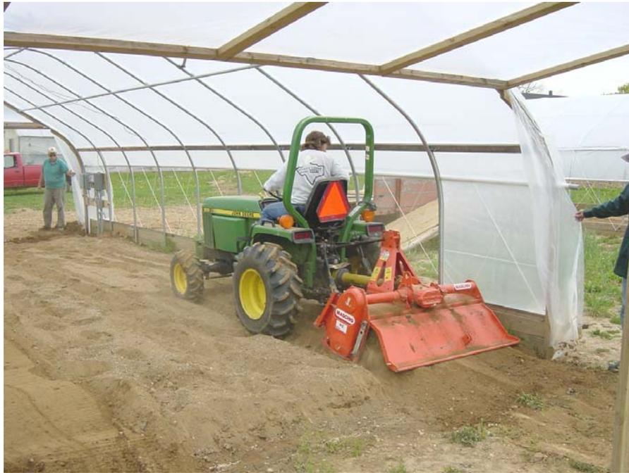
**Photo 3. Soil preparation in a high tunnel using a small tractor.**
