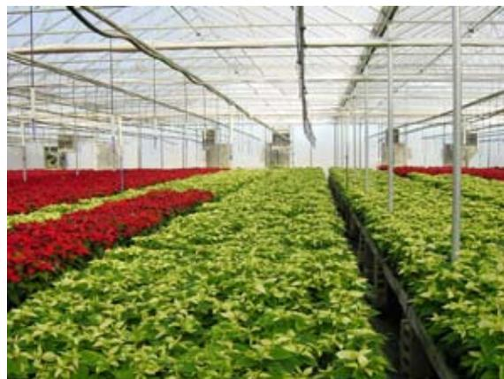
*Figure 2. Multi span, mechanically ventilated greenhouse covered with glass. The plants are grown on benches. The greenhouse is heated using unit heaters. Photo: A.J. Both.*
