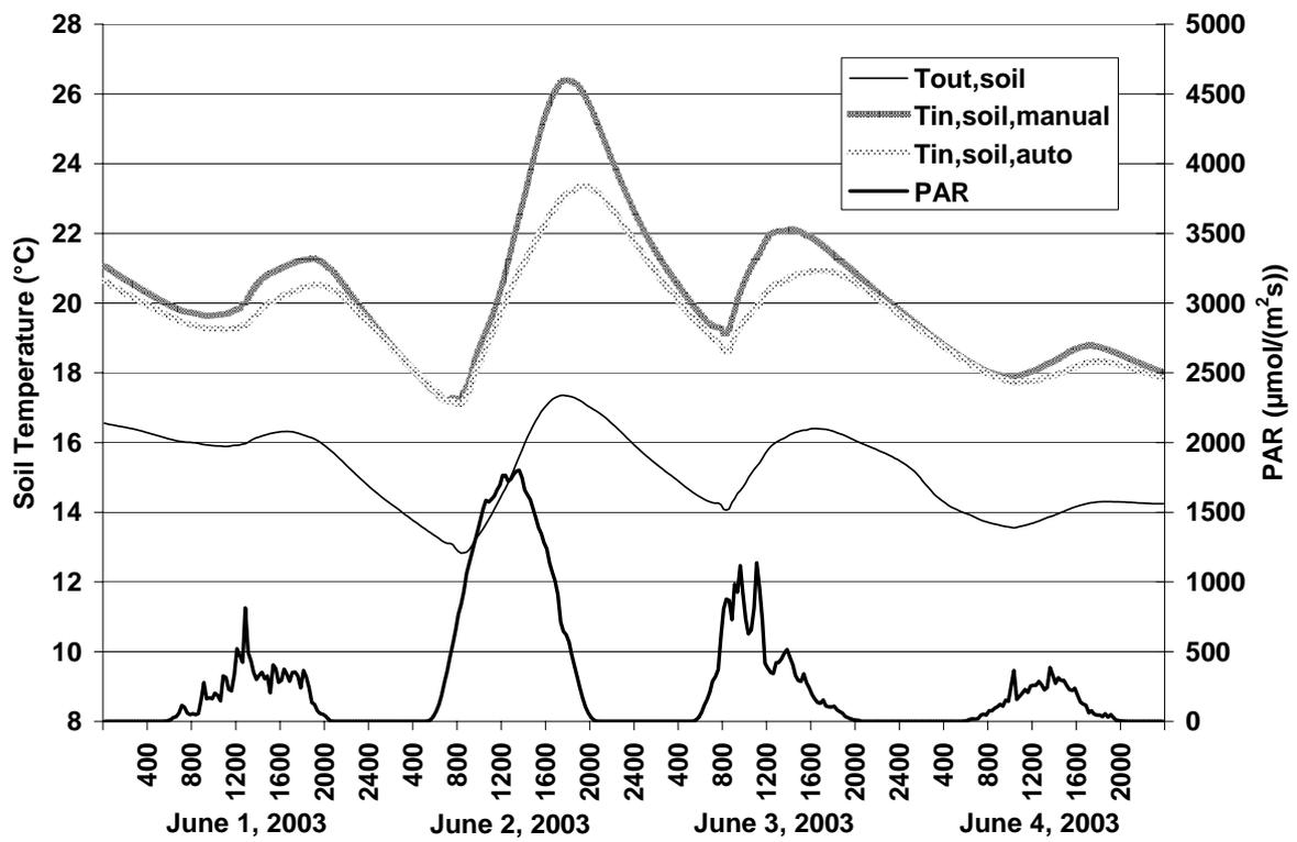
Fig. 7. Measured soil temperatures and outside light intensity (PAR) for June 1-4, 2003.
