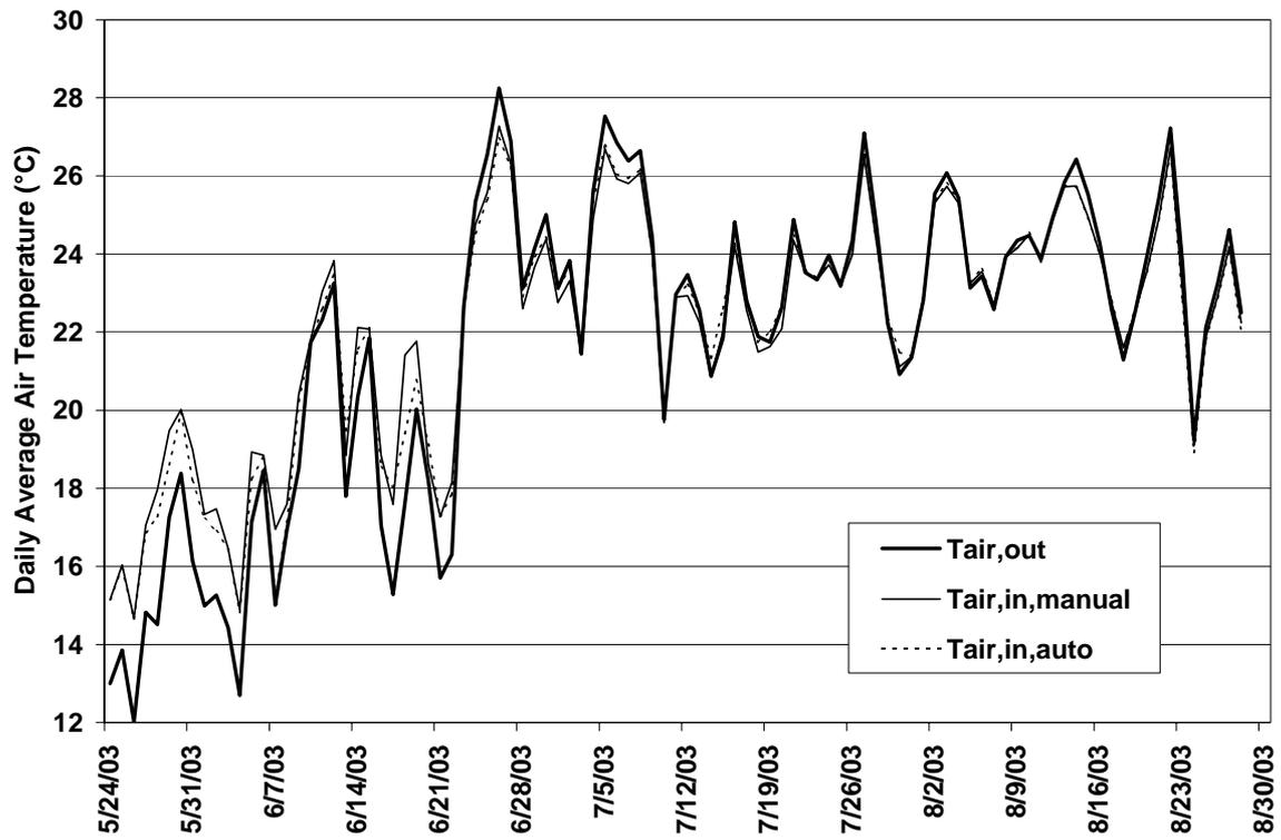
Fig. 4. Measured daily average air temperatures outside and inside the high tunnels.
