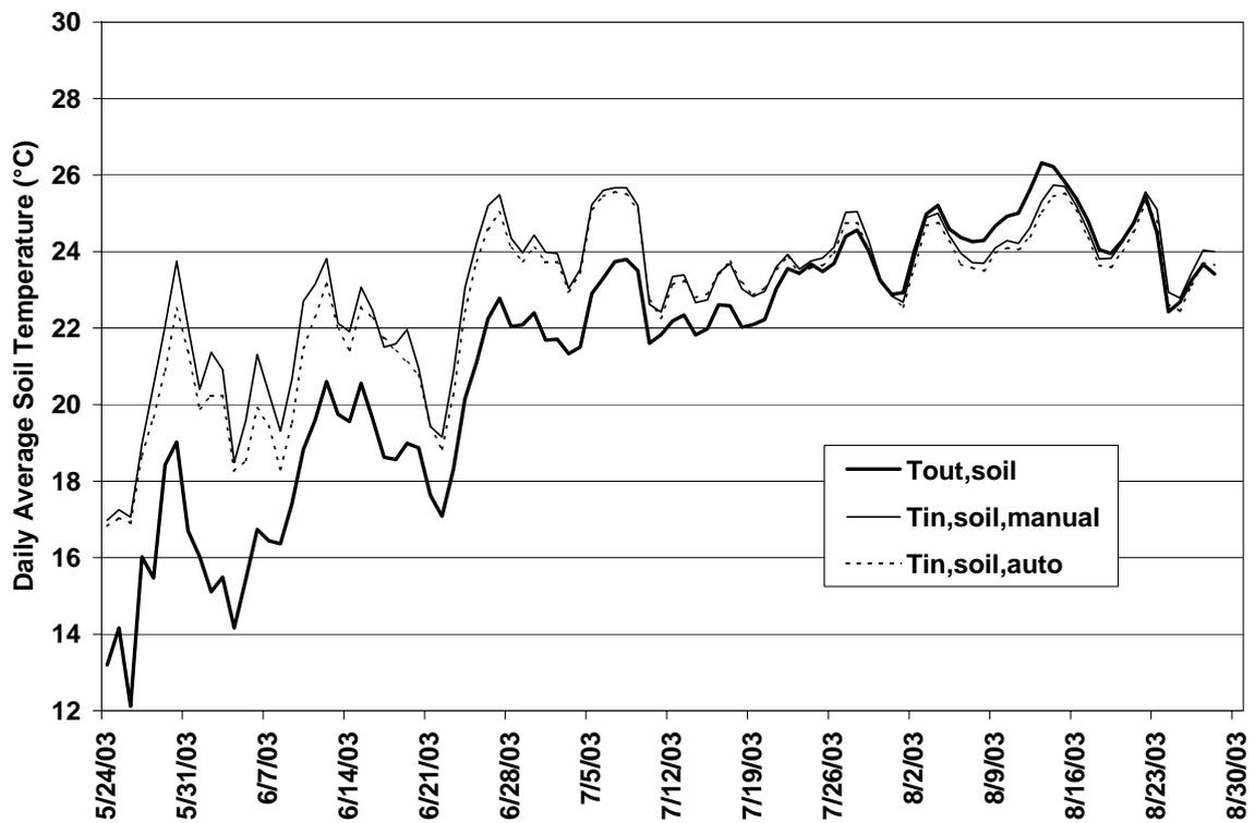
Fig. 5. Measured daily average soil temperatures outside and inside the high tunnels.
